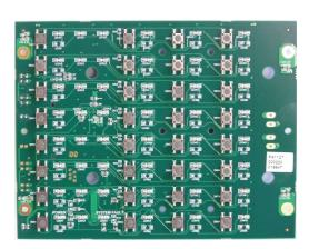
The **QE20-FP2021 Expansion Board** may be used to expand a QE20-FP2013 16 Zone Expander Module if 16 zones are required, or as a replacement for an existing 8 zone board.
